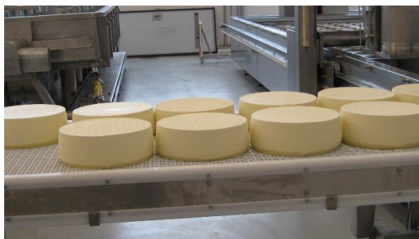
Cheese from the press on the way to the salt brine system
