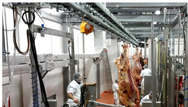
Evisceration line with automatic conveyor system (cattle)
