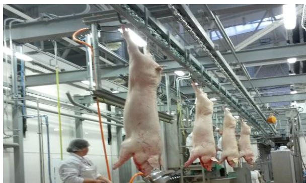
Evisceration line with automatic conveyor system (pigs)
