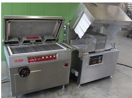
Vacuum packaging and shrinking line
